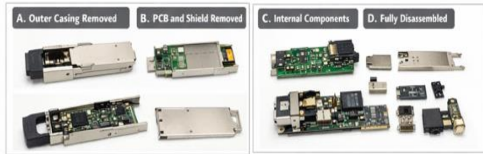
Figure 9: Pluggable Opened Picture: PCB, DSP, optical assembly, and interface connectors
