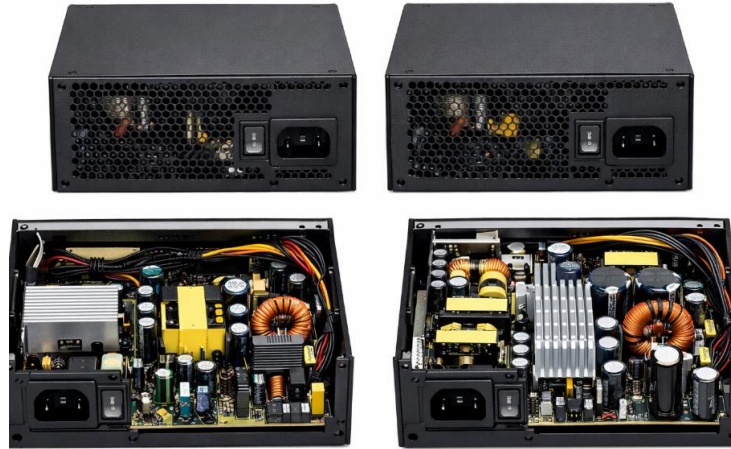
Figure 20: Internally divergent PSU designs with identical external casing.
