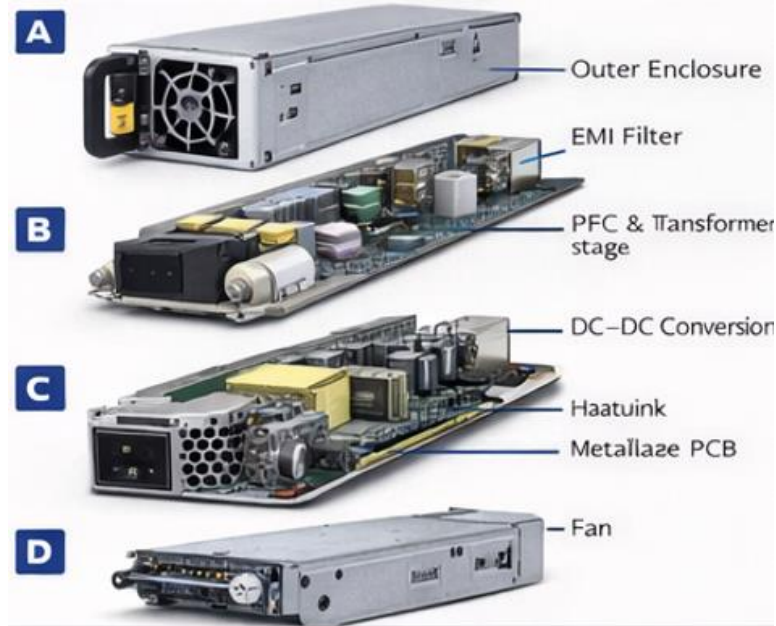
Figure 17: PSU with Enclsure Removed Showing Tear Down Sequence
